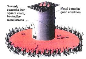
Ground cleared down to mineral soil or gravel at least 10 feet on each side of incinerator
